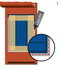
Put a super glue on the edges 9. Put a super glue on the edges of the panel, and place the top fabric on the panel. Remove the tape after the glue is dried.
