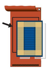
Place the panel and the protection inside of the mark on the fabric and place the top cover on the panel to check the alignment and make sure that the panel cells are not covered by the front fabric.
