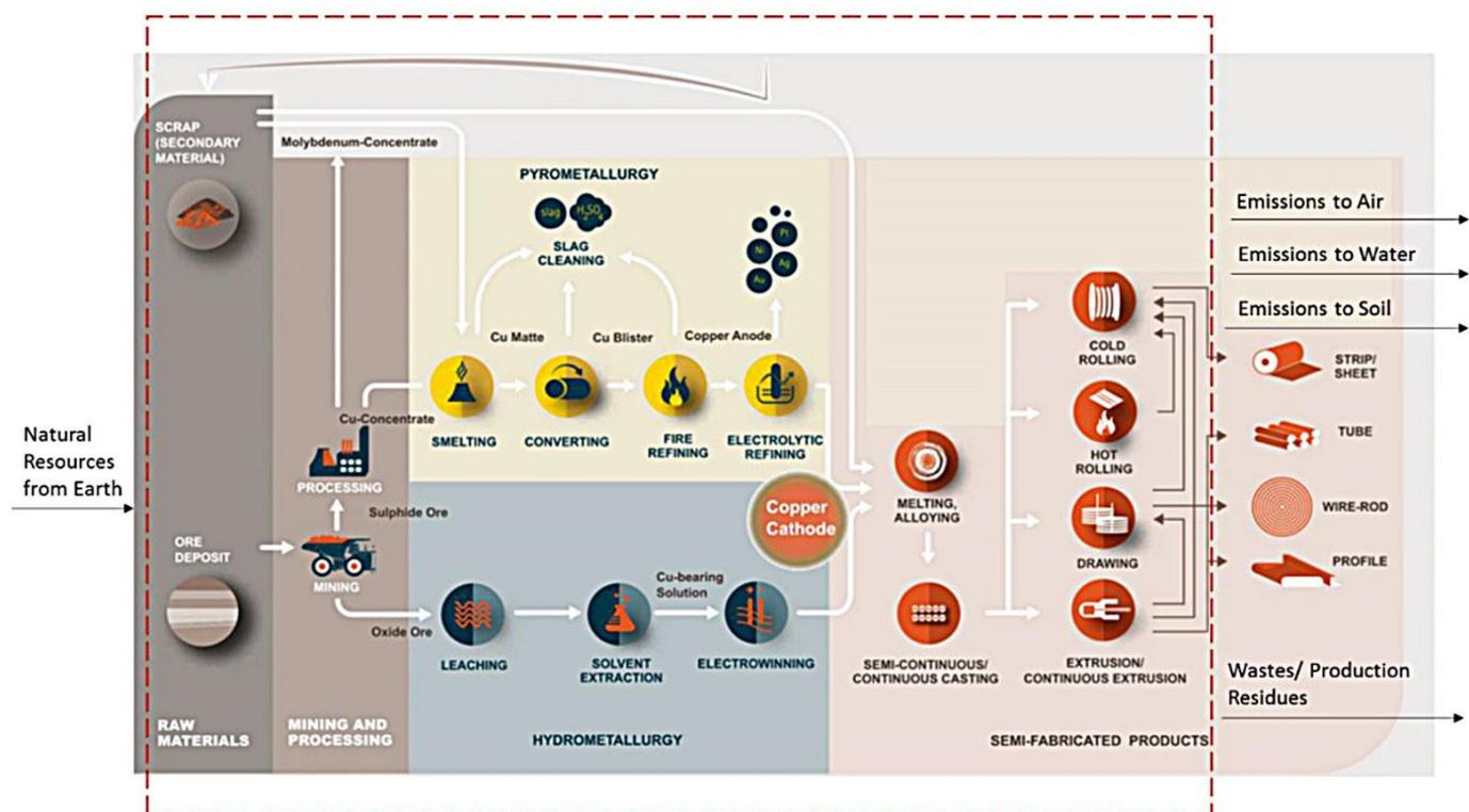
Figure 1. Phases of manufacturing copper products (ECI 2016).
