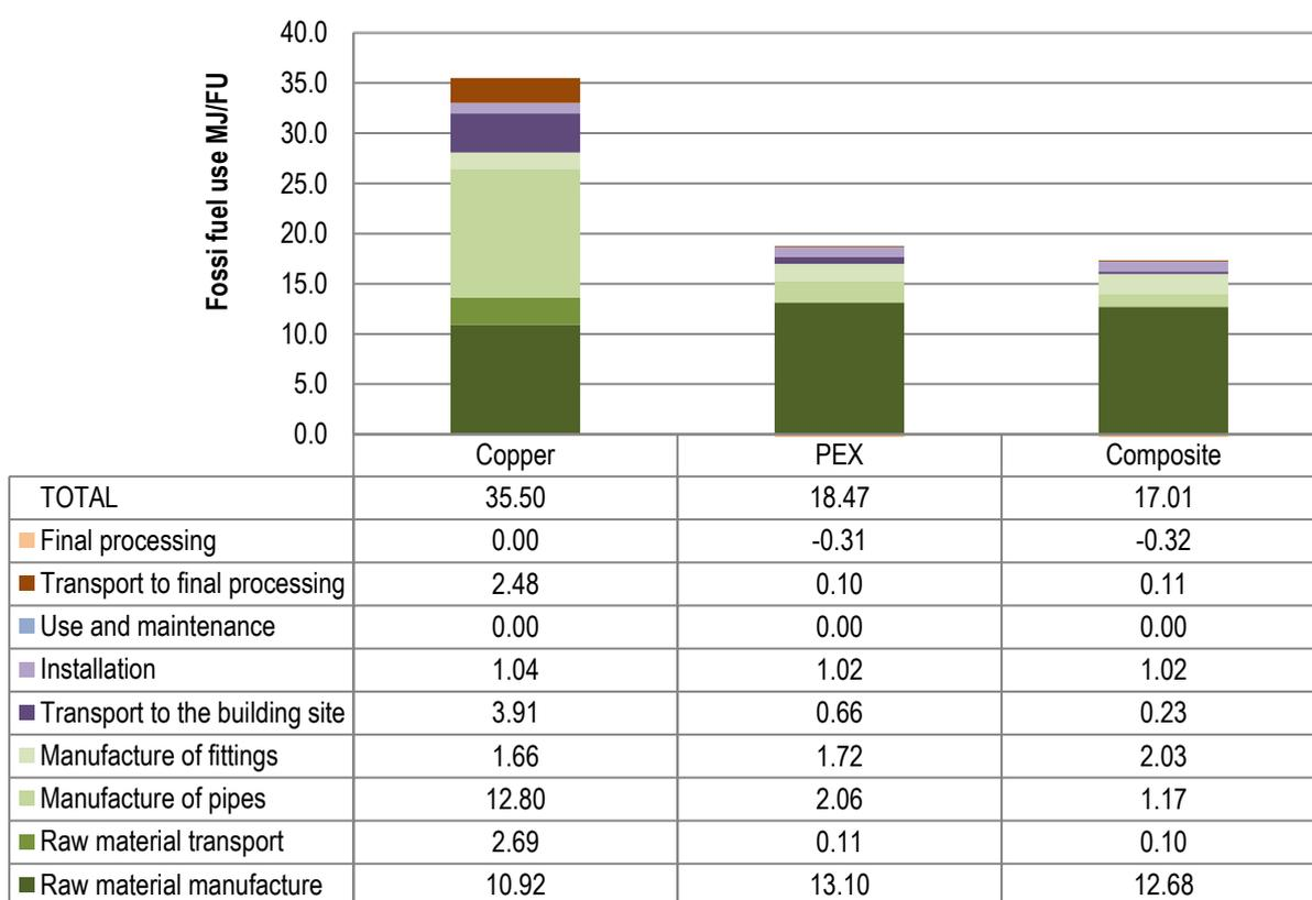
**Figure 3.** The fossil fuel use (MJ) resulting from different pipe materials per functional unit according to assessments by the plastic industry.
