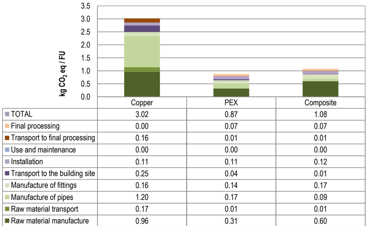
**Figure 2.** The climate change impacts of different pipe materials per functional unit (kg CO<sub>2</sub> equivalent), according to assessments by the plastic industry.
