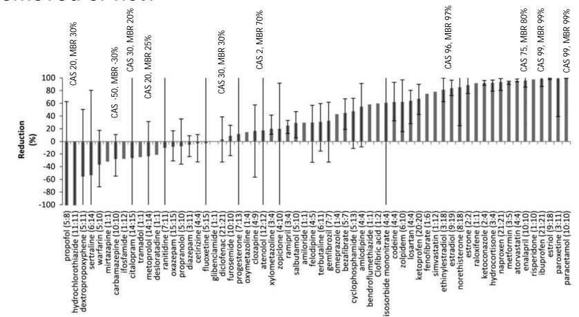
Figure 5 | Median removal efficiency in activated sludge plants with extended nitrogen removal. T-bars indicate standard deviation and numbers within brackets represent – Number of plants used in calculations: Number of plants sampled.
