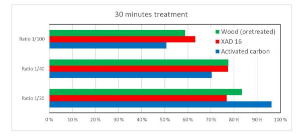
Wood based adsorbents as efficient as activated carbon or polymeric resins
