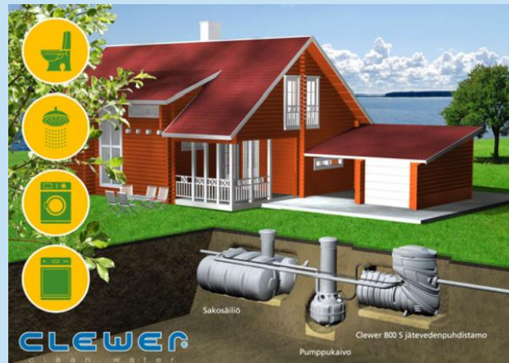
Sedimentation – pumping – biochemical treatment
