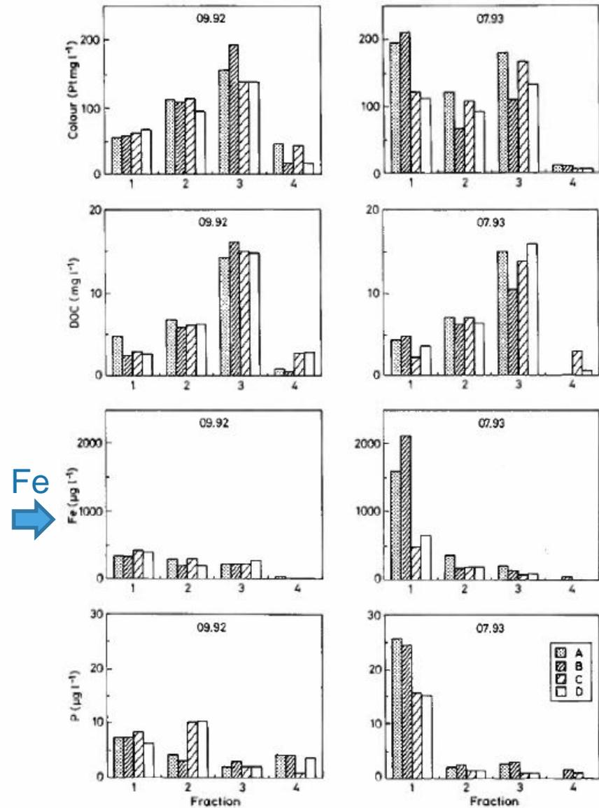
Fig. 4. Colour, DOC, Fe and P in gel filtration fractions  $f_1$ ,  $f_2$ ,  $f_3$  and  $f_4$  from the northern peat mining area of Kompasuo. A = measuring weir above the sedimentation basin and the OFA, B = distribution ditch above the OFA, C = surface water below the OFA, D = measuring weir below the OFA.
