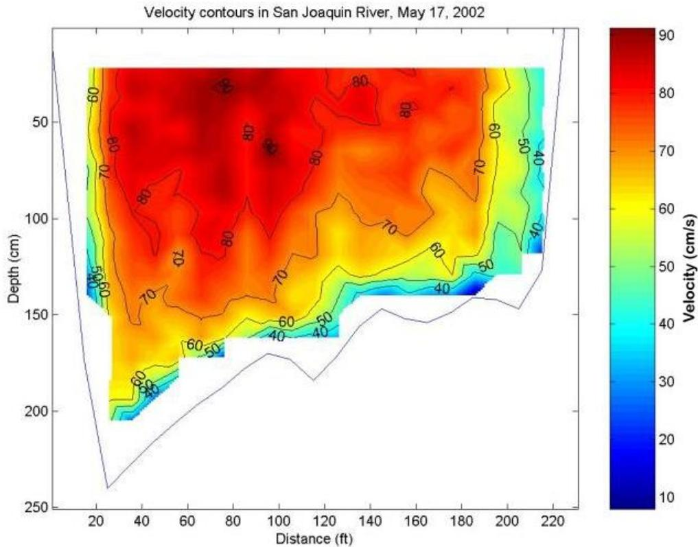
Fig. 4b. An example of the graphical description of a radar-based flow measurement (Cheng et al., 2004).
