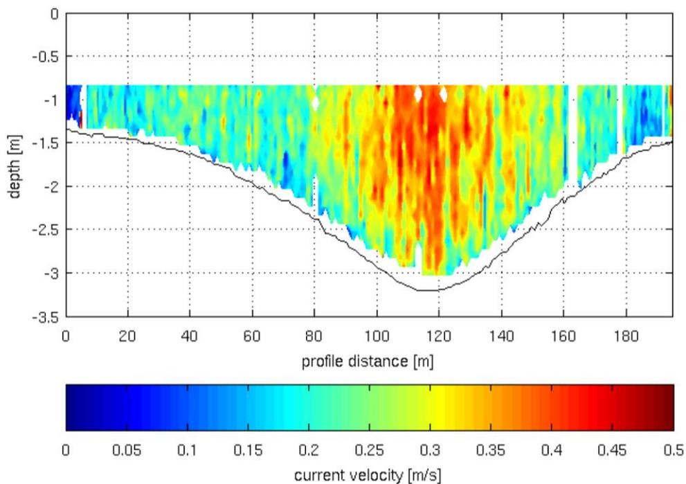
Fig. 3b. An example of the graphical description of an ADCP measurement.
