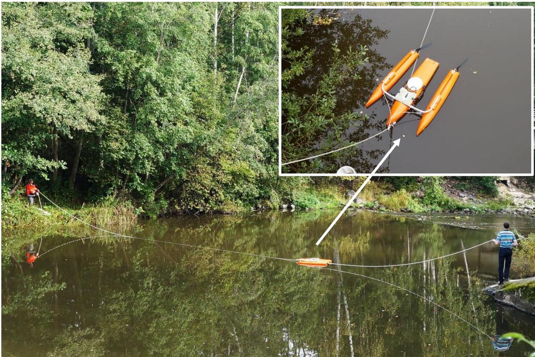
Fig. 3a. An ADCP measurement in a cross-section of the river Vantaanjoki.
