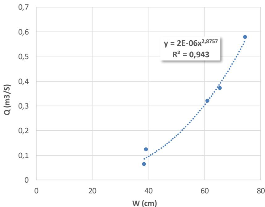
Fig. 5. An example of discharge curve. Water level (W, cm) in the x-axis and the flow rate ( $Q, \text{m}^3 \text{s}^{-1}$ ) in the y-axis. In this case the discharge curve equation is:  $Q = 2 \cdot 10^{-6} \cdot W^{2.8757}$ .
