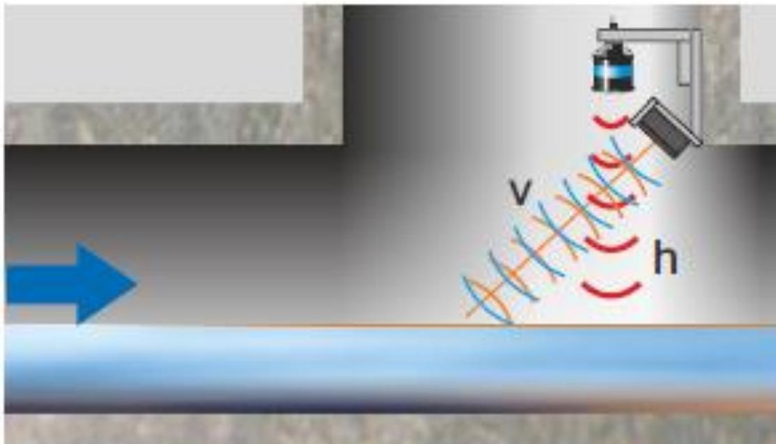
Fig. 4a. The principle of radar flow metering. Two devices measure water velocity ( $v$ ) and height ( $h$ ).
