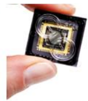
Figure 1. Ion Torrent chip. The grey spherical plates at the outer corners of the outer substrate are 1.4 million wells that sense and record the sequencing reaction.
