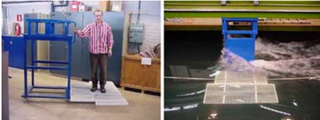
Figure 42 The platform structure (left) fastened to the towing carriage (right).
