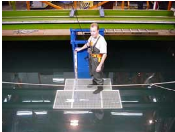
Figure 44 Human subject 3 wearing waders and safety belt. Subject tethered with safety rope.
