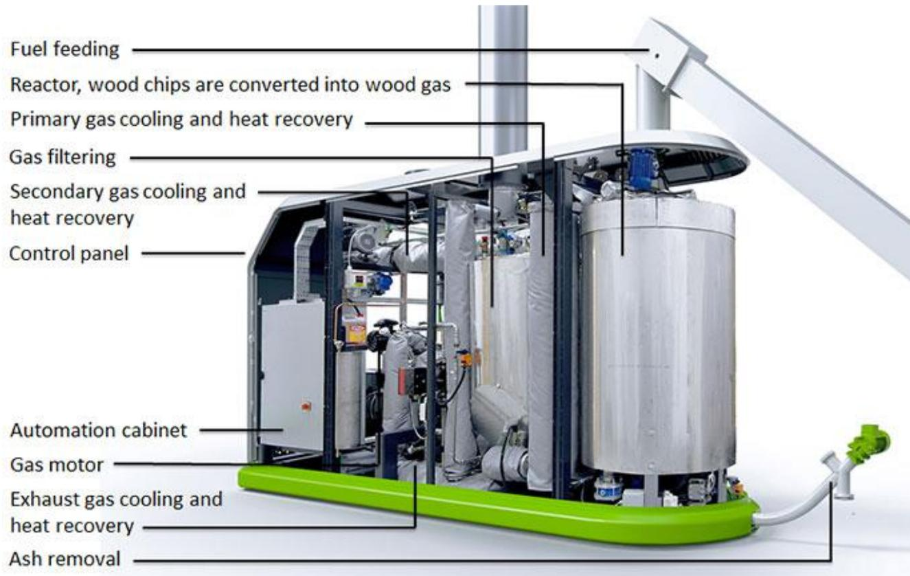
A wood-gasification-based CHP unit from the “eco-village” in Kempele. Source: Volter.
