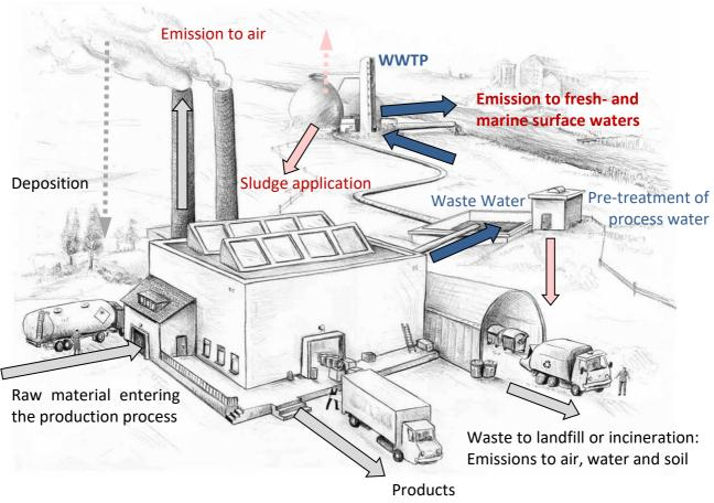
Figure 3: Possible releases from a production process
